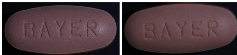
Figure 34. Left: original Stivarga tablet. Right: HPMCAS coated Stivarga tablet. Tablet core size is 16 x 7 mm.
