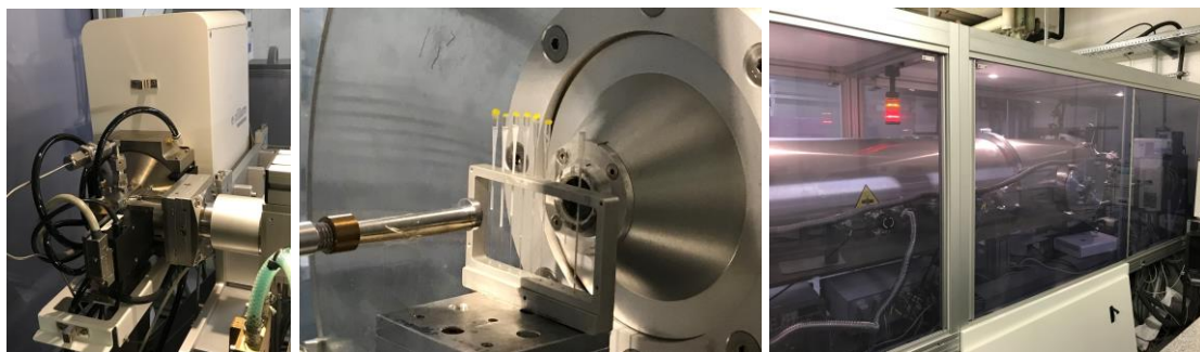
Figure 46. SAXS/WAXS setup at Forschungszentrum Jülich, consisting of X-ray metal jet source (left), capillary autosampler for dissolution samples (middle), and detector tube (right).
