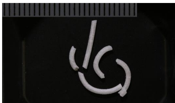
Figure 20. Extrudate RGF_PVP-Witocan 20/80 after extrusion and cooling. The scale bar is in steps of 1 mm.
